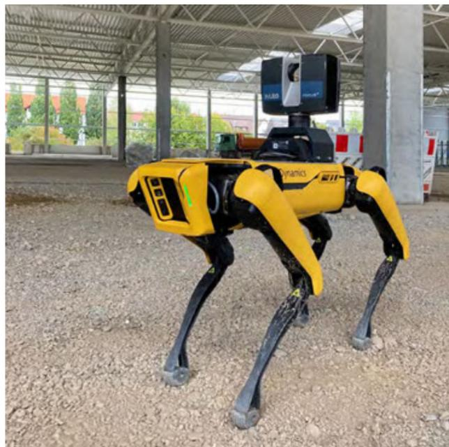
Robot dog Spot created by Boston Dynamics has a 3D laser scanner on its back and has been deployed at GOLDBECK construction sites in Germany as part of a test run.
